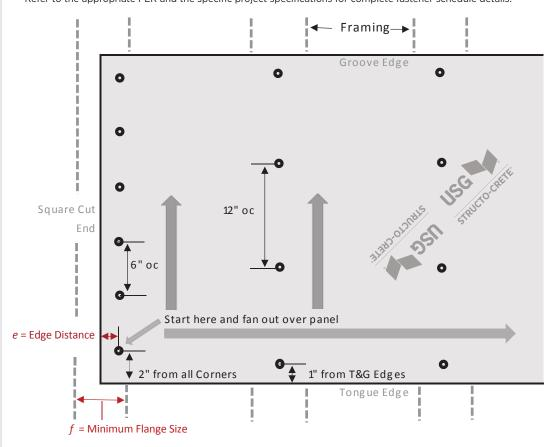
Fastener Quantities: This is intended to be a starting point for fastener estimating only. USG recommends that a calculation be made for each project layout to determine the appropriate number of fasteners required and that an excess of at least 10% be added to the calculated quantity for the project.
